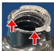
DAMAGED pump retainer ring
