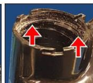
MISSING pump retainer ring
